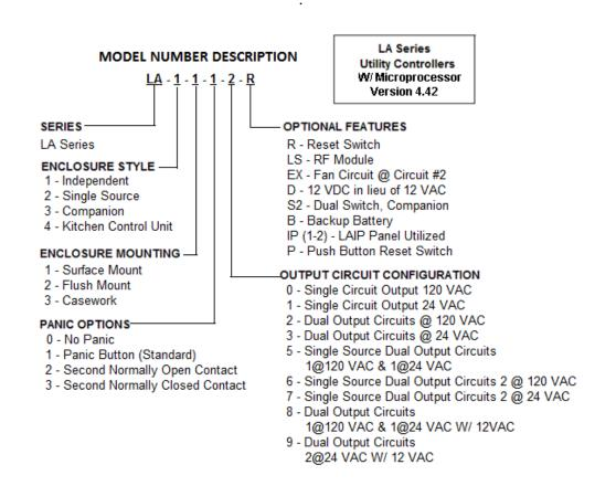
NOTE: Output Configurations 5, 6, 7, 8 and 9 are intended to operate with specific operators and solenoids for applications such as Instructor's Demonstration Stations and Science Preparation Rooms. When Configurations 2 or 3 are specified with Single Source Units, then Outputs are typically provided as single switch operators with or without a Reset per each output.
